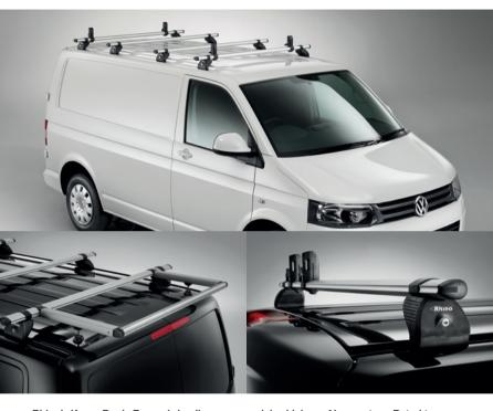
Rhino's KammBar is Europe's leading commercial vehicle roof bar system. Rated to a carry capacity of 75kg per bar, KammBars increase the storage capability of any van considerably, while their contemporary design also adds to the aesthetics of modern commercial vehicles. The system takes its name from Professor Wunibald Kamm, who developed the highly aerodynamic teardrop shape that is seen in the KammBar's aluminium bar profile.
