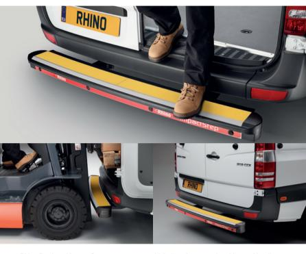
Rhino Products' ImpactStep protects your vehicle from low-speed parking and loading impacts. This significantly reduces body repair costs and vehicle downtime which leads to big savings, particularly across entire fleets. ImpactStep is fitted with advanced shock absorbing units and a special pivoting bracket that protects the vehicle from low-speed impacts to keep your van moving.
